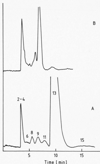
Fig. 2. HPLC elution patterns of carotenes and xanthophylls extracted from A 2 and LHC-II, are shown by curves A and B. The isomer assigned to each peak is given in Table I.
